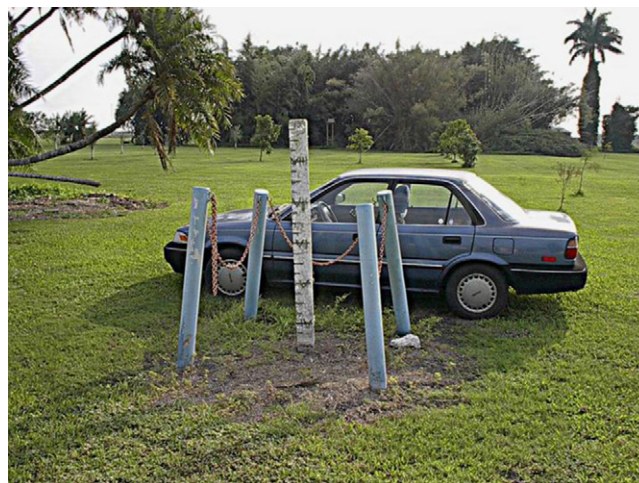
Fig. 3. Subsidence of soil in Florida due to oxidation of organic matter following drainage. When the post was installed in 1923, with its base on bedrock, its top was level with the soil surface. (Photo courtesy of D. Morris, USDA-ARS, Canal Pt. FL.)
